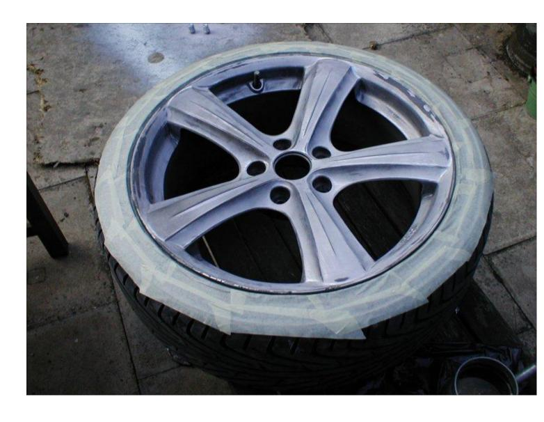
ONCE THE SANDING IS COMPLETE, IT'S TIME TO PRIME THE ALLOY. I JUST USED BODYWORK PRIMER WHICH SEEMED TO DO THE TRICK.
